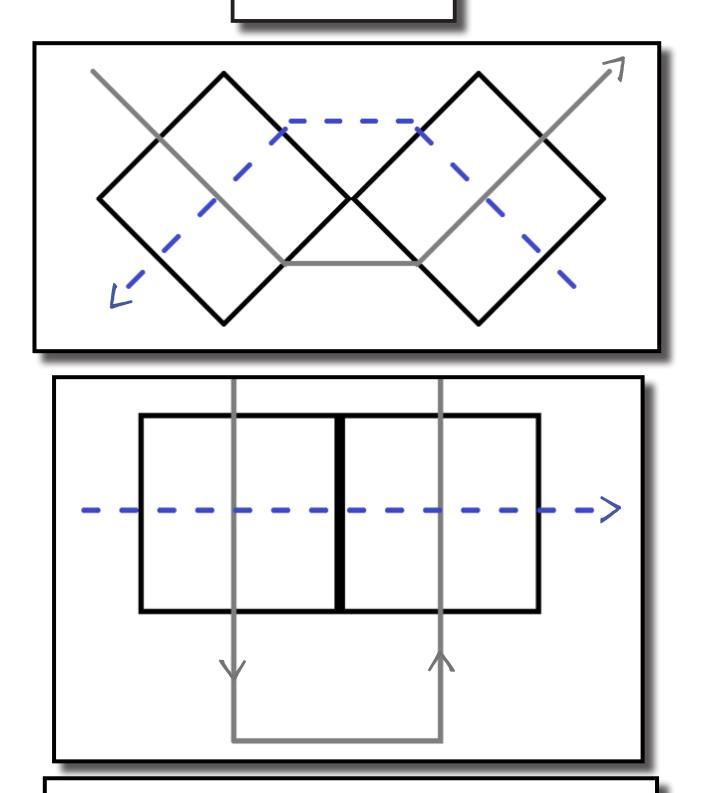
Examples of different configurations on how to arrange multiple Pentagons in cases with need of high capacities. When using larger and vertically standing configurations, the lamellae are supported with seperate load planes.
