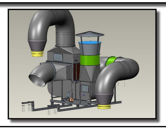
Here is an example of when a rain cap is needed for the exposed channels.
