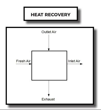
$$\eta = \frac{\text{Inlet air - Fresh air}}{\text{Outlet air - Fresh air}} = \frac{t_i - t_F}{t_o - t_F} \ge 0.93$$
