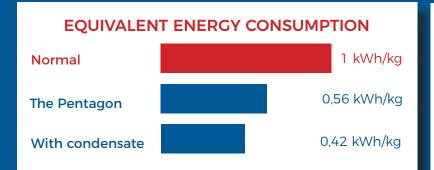
The Pentagon used in the process industry reduces the specific energy from 1 kWh/kg moisture down to 0,56 kWh/kg moisture. If it is possible to use the condensate we are able to reach 0,42 kWh/kg moisture.
