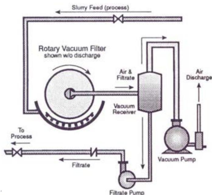
cylindrical surface is covered by a **filter cloth** with a mesh size appropriate for the sludge characteristics.
