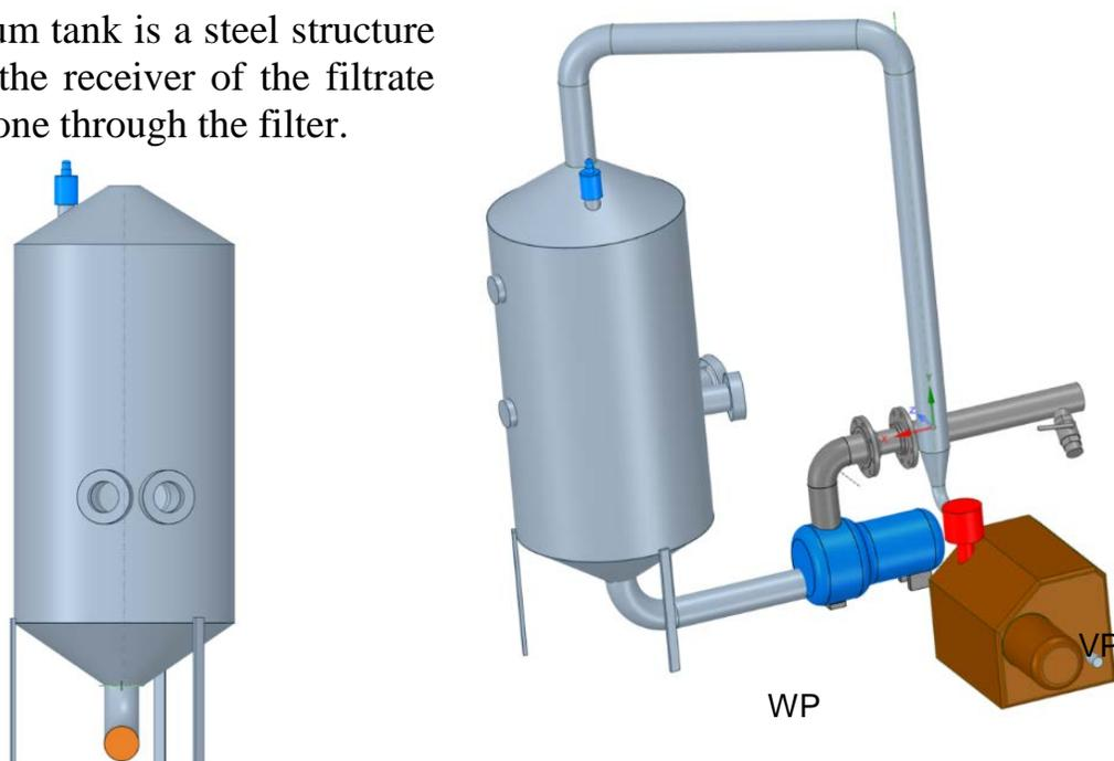
The top and bottom pipes on the cylindrical surface linked to the drum are for the air and water flows respectively. The pipe on the top cone is connected to the vacuum pump, while the one at the bottom cone is connected to the water pump.
