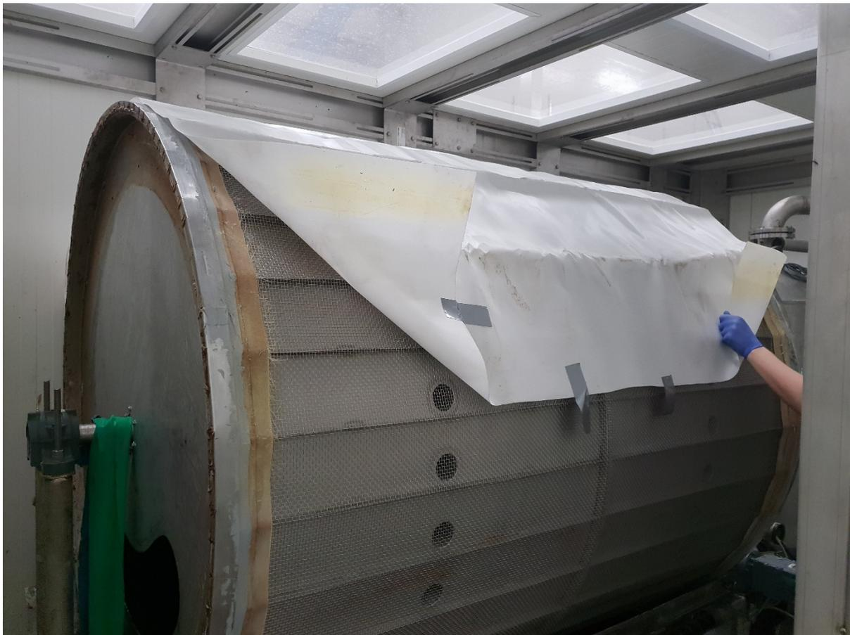
*Figure 8: Pictures of the drum without and the cloth and during installation*
