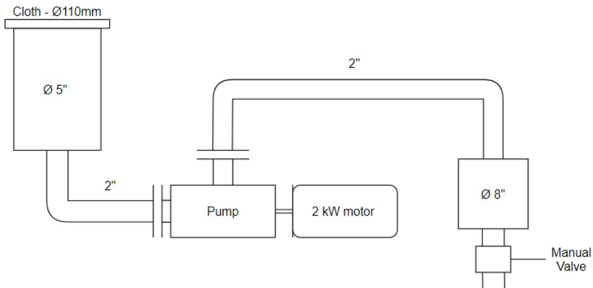
*Figure 9 Schematic representation of the test experiments*
