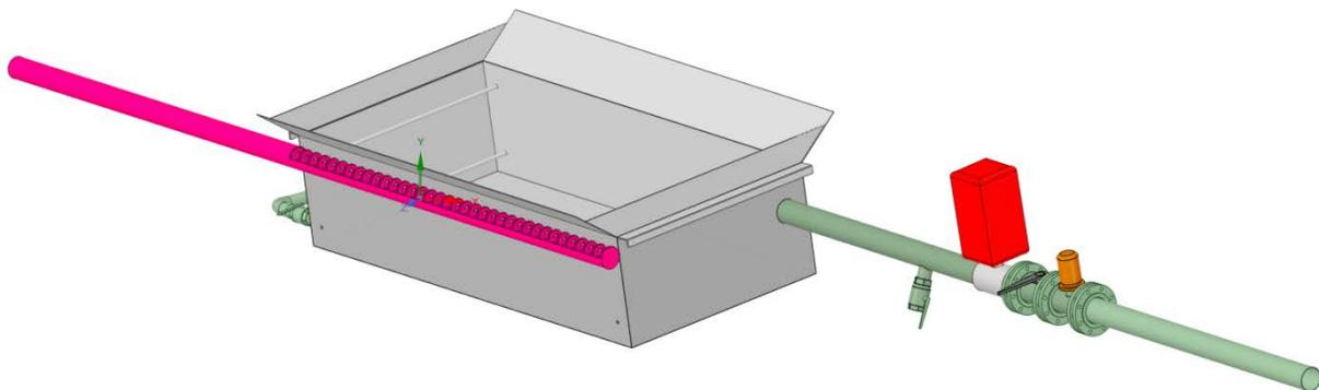
The sludge tank is a stainless steel tank used to contain the sludge in which the drum is immersed, as well as supporting the drum. The inlet pipe is equipped with a regulating valve, in red in the drawing above. A draining outlet, present on the back side of the tank, can be used to empty and clean the tank. The tank also includes 1600 inclined transversal steel tubes used for condensation.
